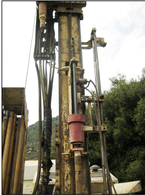
Figure 15: Automatic trip SPT hammer used in DCPT probing.
