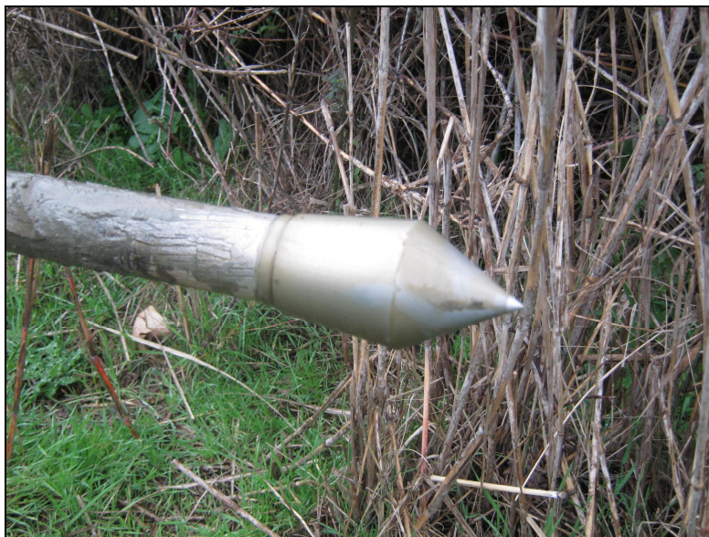
Figure 13: Solid cone used in DCPT
