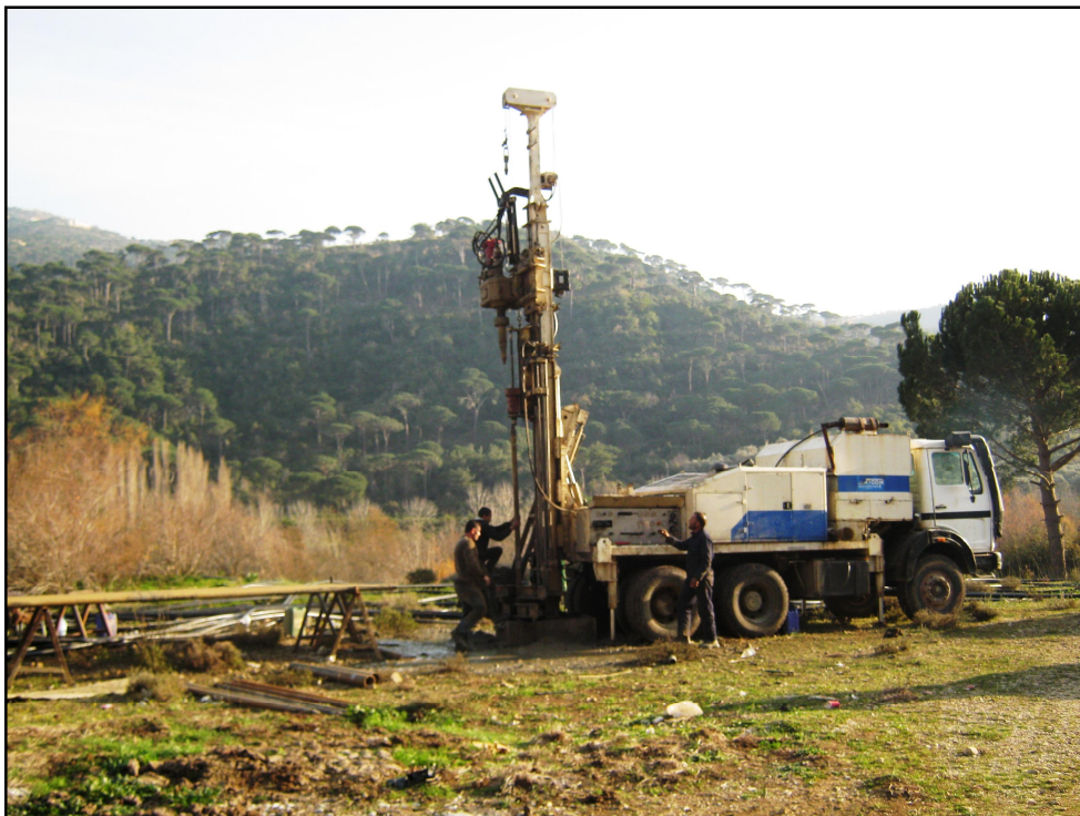
Figure 9: Truck mounted drill rig used in DCPT probing.
