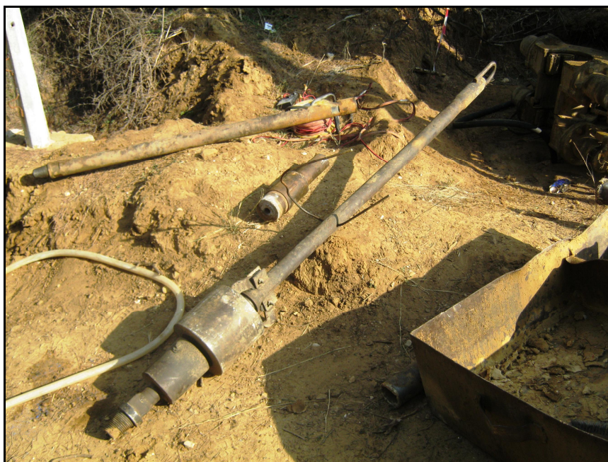
Figure 14: Automatic trip SPT hammer used in boreholes.
