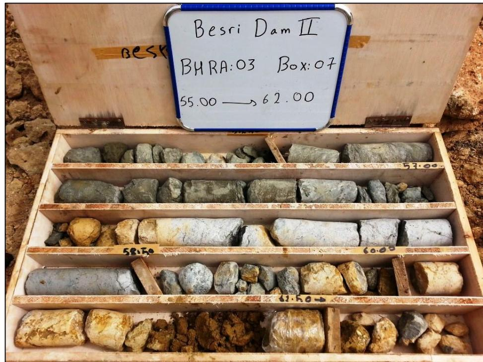
Figure 11: Standard wooden core boxes
