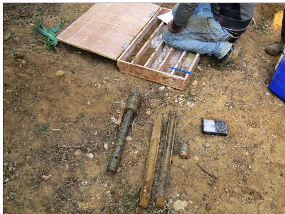
Figure 12: SPT sampler
