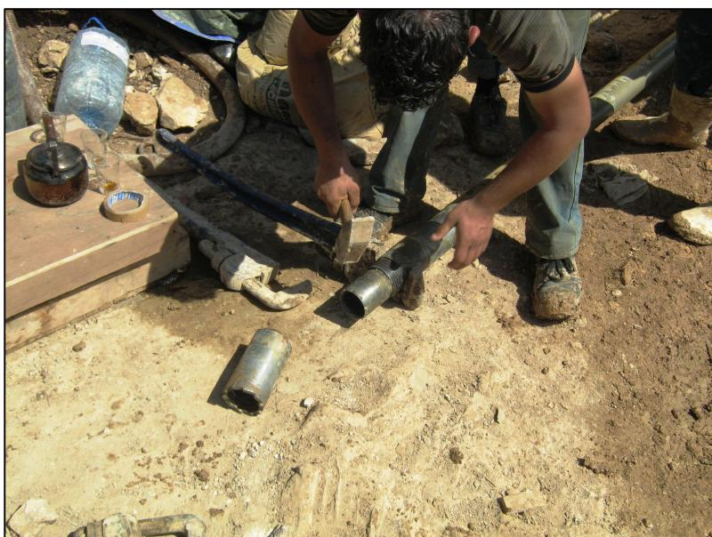
Figure 10: Double tube core barrel
