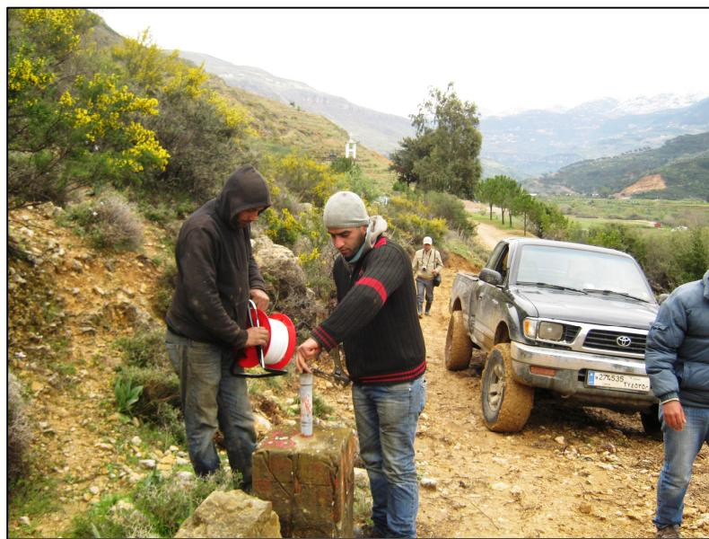
Figure 20: Measuring the depth of groundwater
