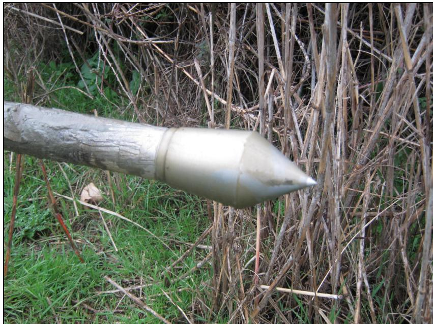
Figure 13: Solid cone used in DCPT
