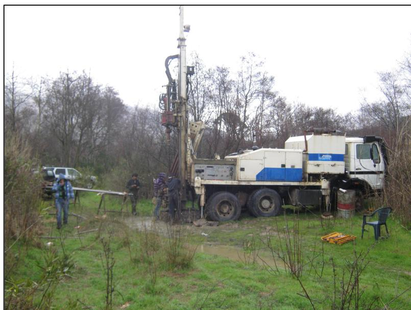
Figure 16: Continuous DCPT probing.
