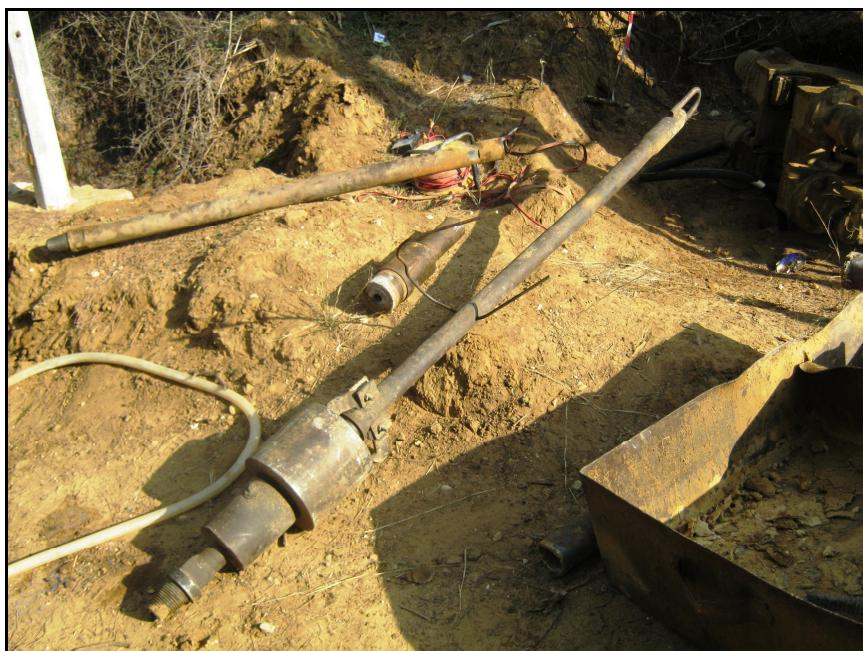
Figure 14: Automatic trip SPT hammer used in boreholes.
