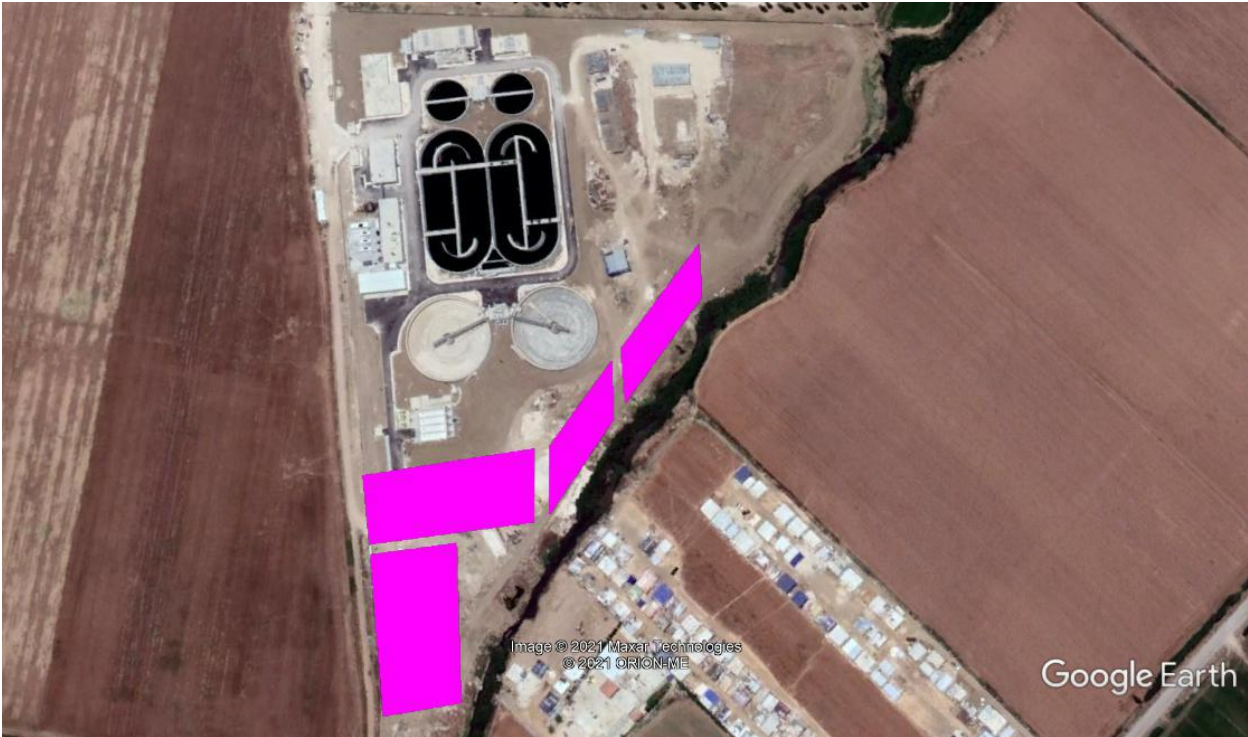
General Layout of the solar dryers in Zahlé at the 2040 horizon (scenario 4)
